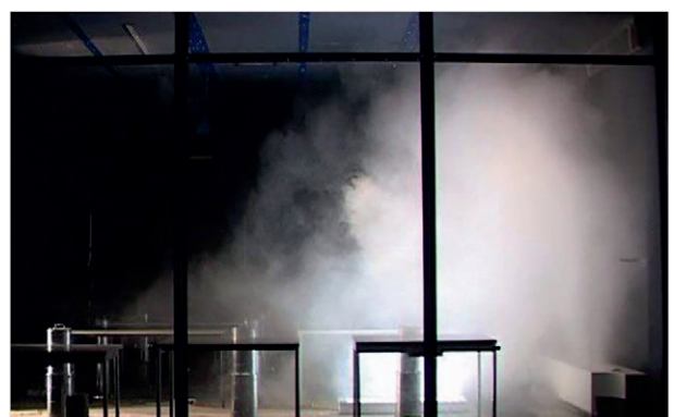
Example of room air flow VFC-N with special fan insert for mixed/displacement air
