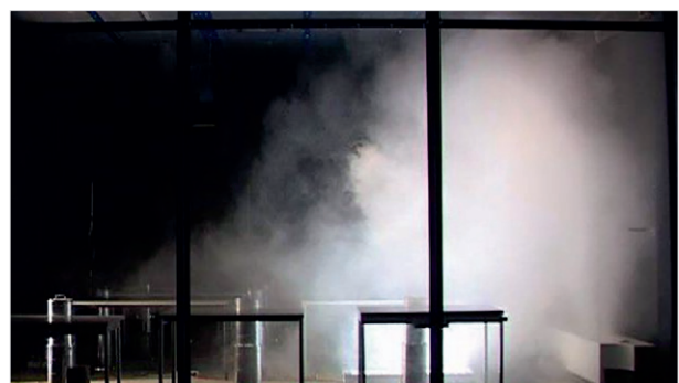
Example with special fan insert for mixed/displacement flow
